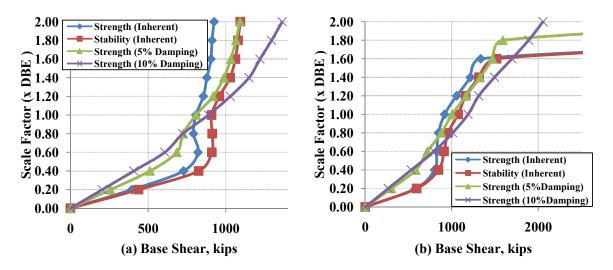
Figure 4 Base Shear IDA Plots for Erzincan (a) and Miyagi Oki (b) Earthquakes
