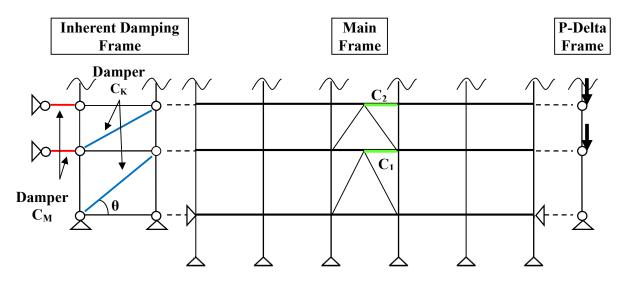
Figure 1. Inherent Damping and P-Delta Frames Constrained to Main Frame
