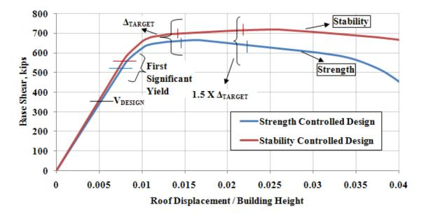
Figure 2. Nonlinear static pushover curves for strength and stability controlled designs
