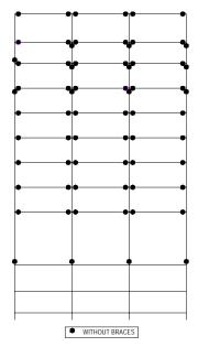
Figure 6. Plastic hinges global distribution, C axe (transversal direction) without braces
