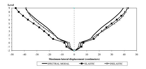
Figure 5. Maximum lateral displacements, C axe (transversal direction) without braces
