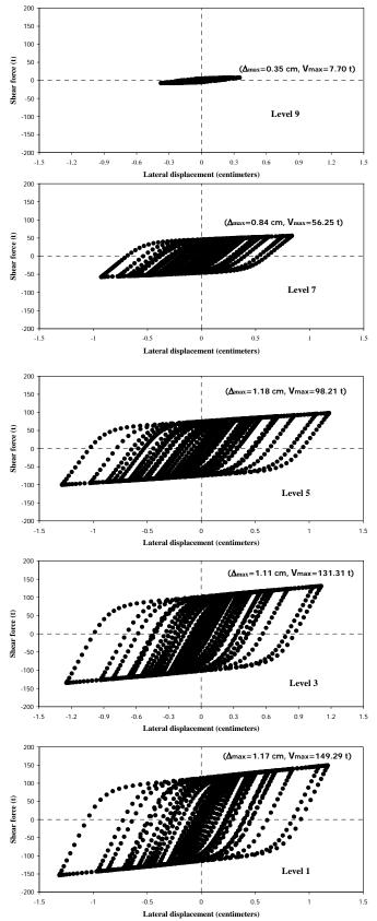
Figure 9. Ratios of shear force-lateral displacement of energy dissipation elements in levels 9, 7, 5, 3 and 1
