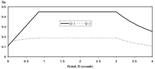
Figure 2. Design spectra, seismic zone III<sub>b</sub>, Q=1 y Q=3, Mexico City Code (RDF-04)
