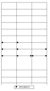
Figure 8. Plastic hinges global distribution, C axe (transversal direction) with braces
