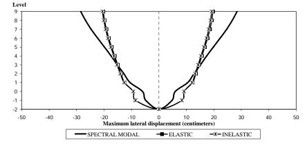
Figure 7. Maximum lateral displacements, C axe (transversal direction) with braces
