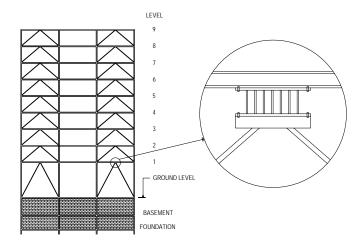
Figure 1.b Transversal direction frame, model 2 (with braces and ADAS)
