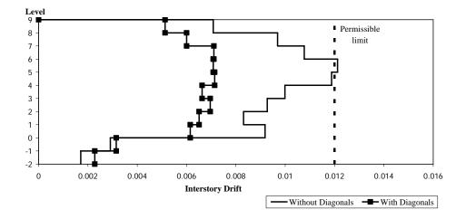
Figure 3. Ratios of relative lateral displacement between the story-height ( $\Delta r_i/h_i$ ), earthquake in direction X
