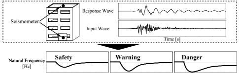
Figure 1 The application for structural health monitoring by using the transient change of natural frequency.
