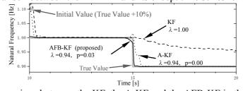
Figure 7 Comparison between the KF, the A-KF and the AFB-KF in the STEP type.
