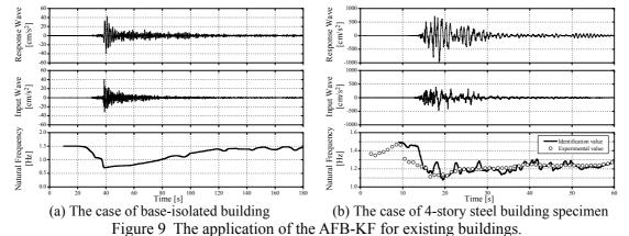
load-displacement relationship is calculated from the records of both absolute acceleration and relative story displacement on every story, and the transit change of natural frequency of experimental building during shaking test is calculated by performing eigenvalue analysis from the load-displacement relationship and weight of every story. In Figure 9(b), the experimental value of natural frequency calculated by this way is also shown.
