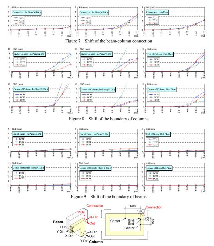
Figure 10 Definition in direction of each shearing and the measurement locations
