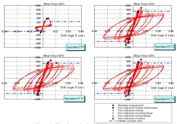
Figure 6 Shear force – horizontal deformation relationships
