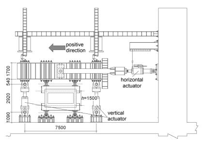
Figure 3 Dynamic loading apparatus
