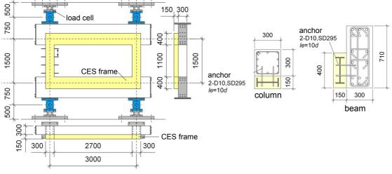
Figure 2 Test specimen
