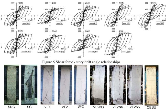
Photo 1 Crack modes of specimens after loading
