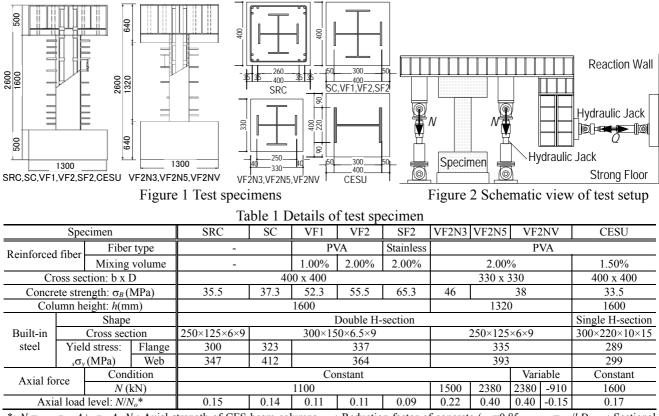
\*:  $N_o = {}_{c}r_u \cdot \sigma_B \cdot {}_{c}A + {}_{s}\sigma_y \cdot {}_{s}A$ ,  $N_o$ : Axial strength of CES beam-columns,  ${}_{c}r_u$ : Reduction factor of concrete ( ${}_{c}r_u = 0.85 \cdot {}_{s}p_c, {}_{s}p_c = {}_{s}a_c/bD$ ,  ${}_{s}a_c$ : Sectional area of steel flange on compressive side),  ${}_{c}A$ : Sectional area of concrete,  ${}_{s}A$ : Sectional area of Steel
