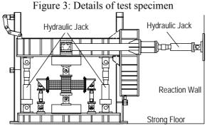
Figure 4 Schematic view of test setup
