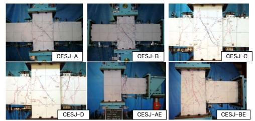
Photo 2 Crack modes of specimens at R of 0.03rad.
