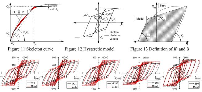
Figure 14 The comparative results of shear force-story drift angle relationship
