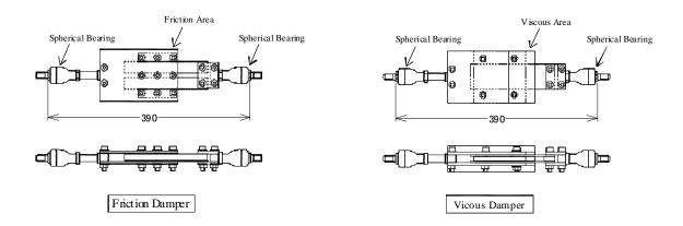
Figure 2. Schematic diagram of friction damper
