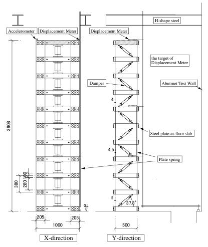
Figure 1. Schematic diagram of test subject
