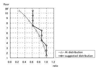
Figure 4. Vertical damper quantity ratio
