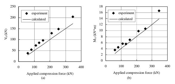
Figure 3.4 Relationship between applied compression force,  $V_0$  and  $M_0$
