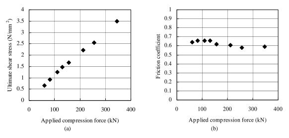
Figure 3.2 Ultimate shear stress and friction coefficient
