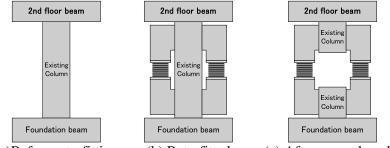
(a)Before retrofitting (b) Retrofitted (c) After an earthquake Figure 1.1 concept of the soft-landing base-isolation system
