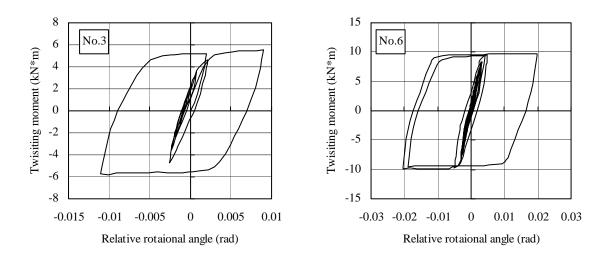
Figure 3.3 Relationship between relative rotational angle and twisting moment
