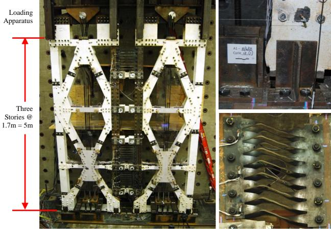
Figure 4 Half Scale Test Setup at UIUC (Left), Uplifted Base Connection (Top Right), Deformed Fuse (Bottom Right)
