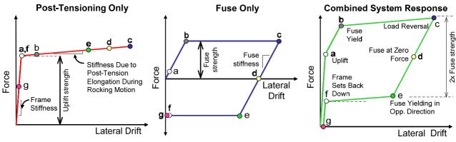
Figure 2 Schematic Depiction of the Controlled Rocking Hysteretic Response
