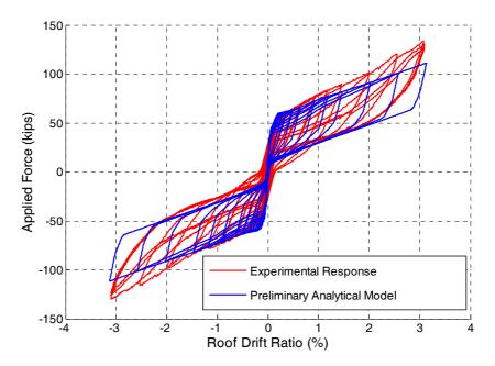
Figure 7 Comparison of the Experimental Results and the Preliminary Analytical Model
