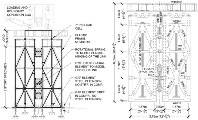
Figure 6 Schematic Representation of the OpenSees Analytical Model (Left) and Specimen Geometry (Right)
