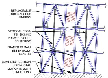
Figure 1 Controlled Rocking System (Left) and the Analytical Model Created In OpenSees (Right)
