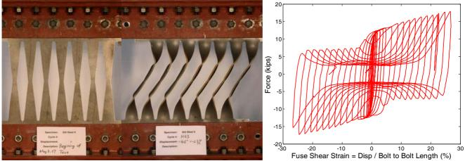
Figure 3 Undeformed Fuse (Left), Fuse at 23% Shear Strain (Middle), and Fuse Hysteretic Response (Right)
