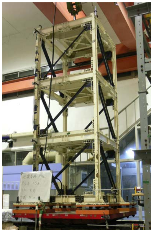
Figure 4 TFPS Isolated structure on the shaking table
