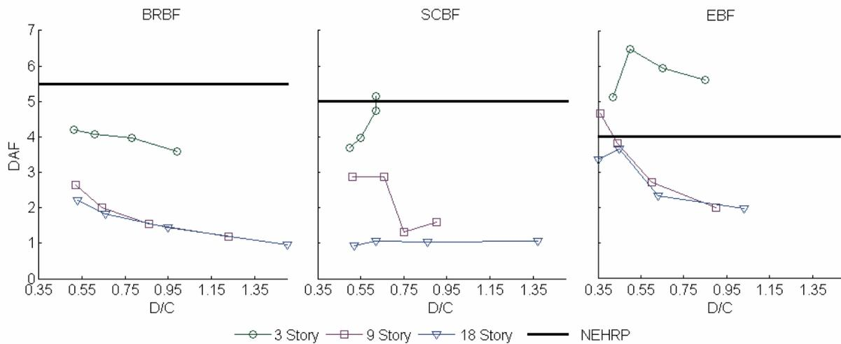
Figure 2 Roof Drift DAFs
