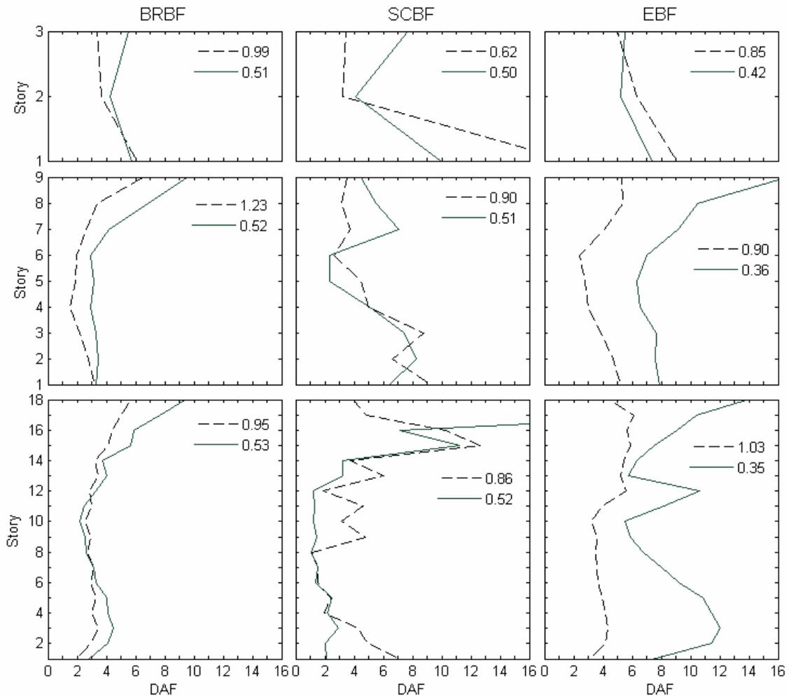
Figure 4 Shear Interstory Drift by Floor
