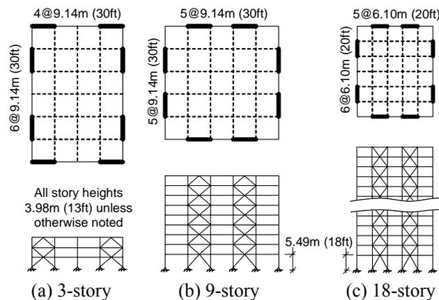
Figure 1 Plan and elevation views of SCBF and BRBF buildings
