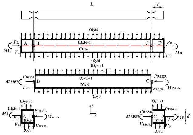
Figure 4 Free body diagram of intermediate HBE
