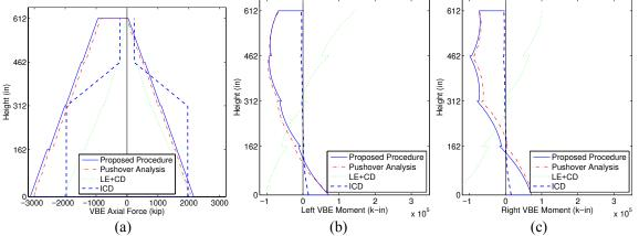
Figure 4 Design Actions for SPSW-C VBEs (a) Axial Force (b) Left VBE Moment (c) Right VBE Moment
