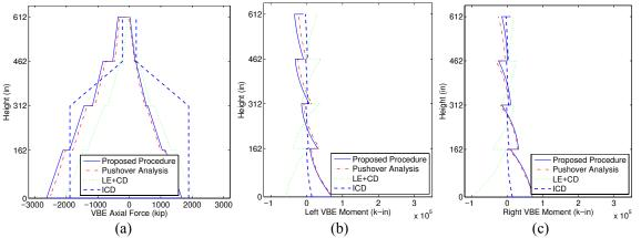
Figure 5 Design Actions for SPSW-V VBEs (a) Axial Force (b) Left VBE Moment (c) Right VBE Moment
