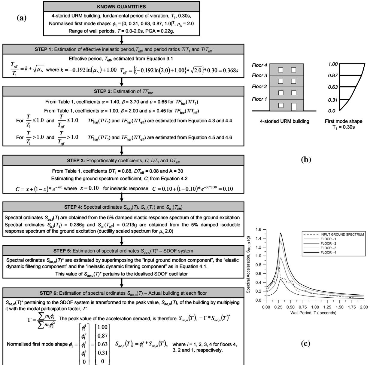
Figure 6: (a) Procedure for estimating floor acceleration demands in an example 4-storied URM building, shown in (b) and (c) floor acceleration spectra for floors 1-4 of the URM building
