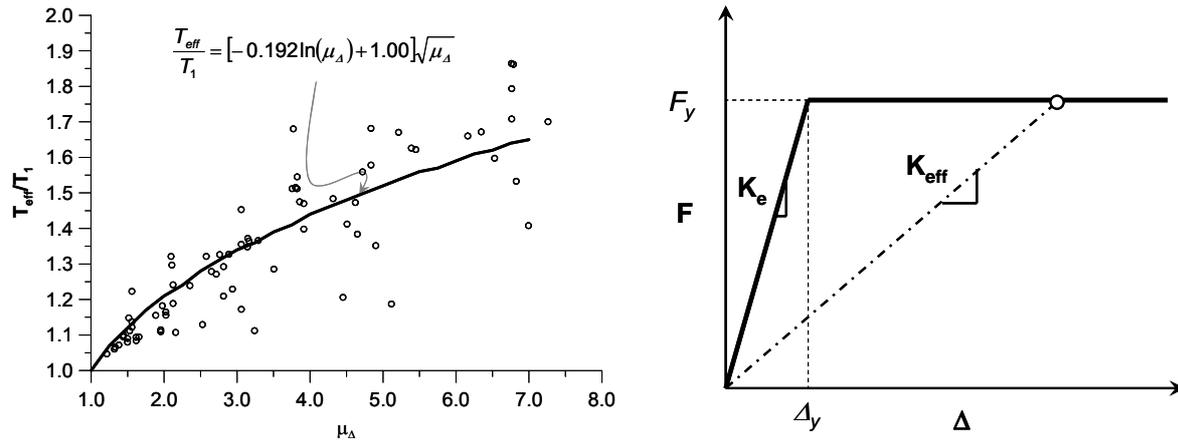
Figure 4: (L) Semi-empirical equation relating the period ratio ( $T_{eff}/T_1$ ) to  $\mu_{\Delta}$  obtained by regression analysis of inelastic THA (each point represents average of 10 THA); (R) Secant stiffness approach
