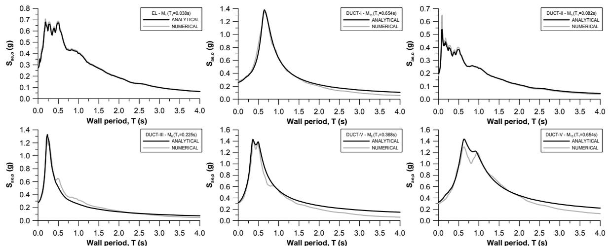
Figure 5: Comparison of acceleration demands computed using the proposed expression with THA results for different oscillators under elastic and ductile response (ductility classes – refer Table 1)
