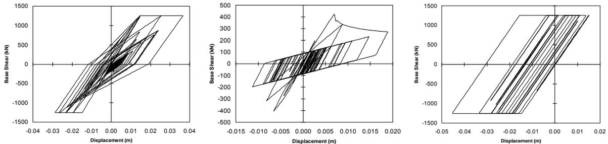
Figure 1: Hysteresis response of the SDOF oscillator representing the primary system using (left) modified-Takeda; (centre) masonry shear-dominated; (right) EPP hysteretic rules
