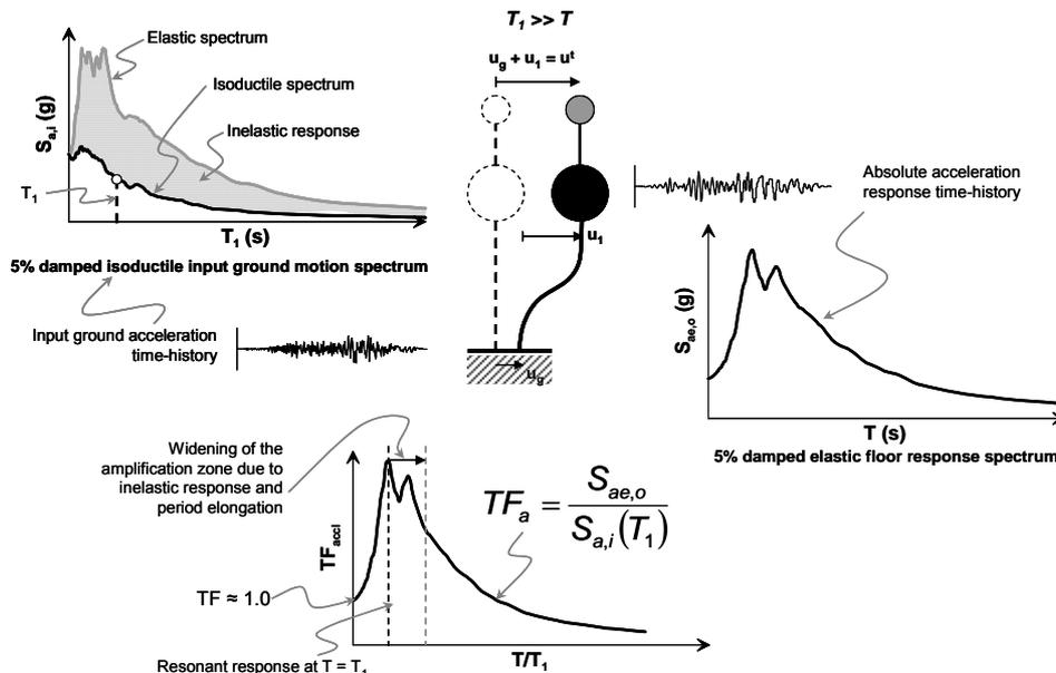
Figure 2: Acceleration transfer function for a flexible primary structure under inelastic response
