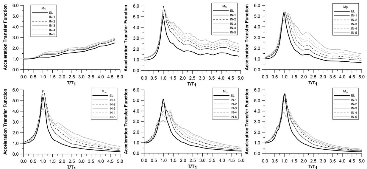
Figure 3: Acceleration transfer functions for all target  $\mu_A$  for oscillators  $M_1$  ( $T_I=0.04s$ ),  $M_4$  ( $T_I=0.12s$ ),  $M_6$  ( $T_I=0.23s$ ),  $M_{10}$  ( $T_I=0.48s$ ),  $M_{14}$  ( $T_I=0.72s$ ) and  $M_{17}$  ( $T_I=0.95s$ ).
