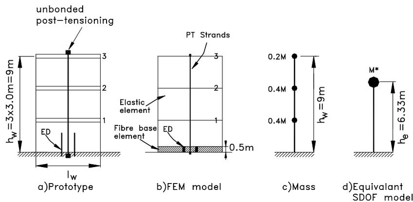
Figure 4-Prototype wall and modeling
