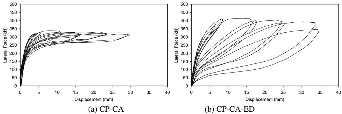
Figure 3-Force-displacement response
