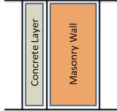
Figure 5 The basic cell of retrofitted masonry
