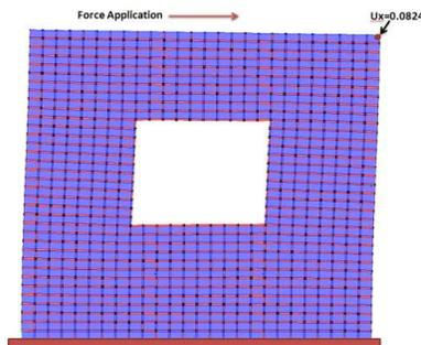
Figure 4 The deformed shape of the micro model under in-plane load
