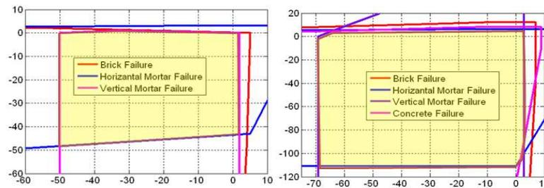
Figure 6 yield surface of homogenized masonry(left) and retrofitted masonry(right)
