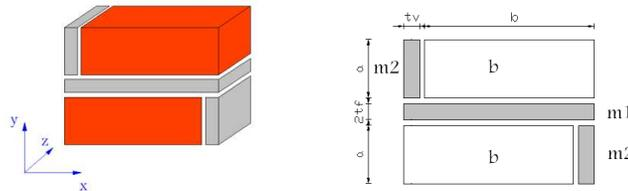
Figure 2 The dimensions of the basic cell's constituents
