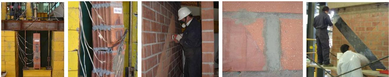
Figure 2 Bond test, surface preparation and CFRP bonding.
