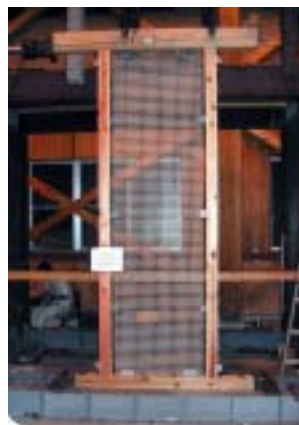
Figure 5 Bearing Wall of Half Opening Rate
