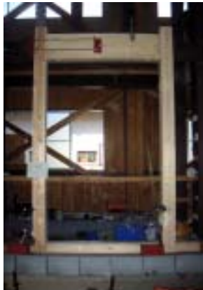
Portal Frame n=2.15/\text{Frame} (Experiment)
