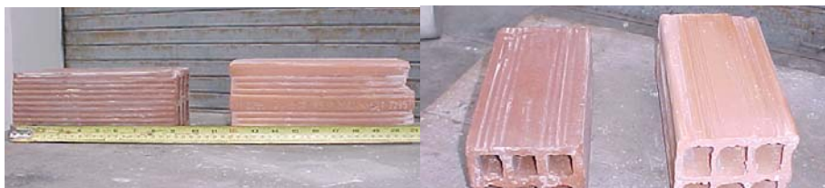
Figure 2. Tubular masonry bricks. Non standard (left) and Standard (right).
