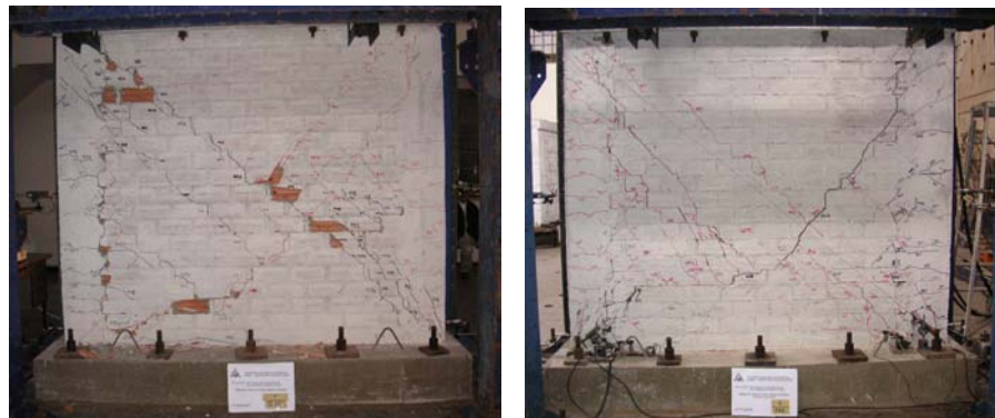
Figure 4. Final condition of walls. Left: S-masonry. Right: U-masonry.
