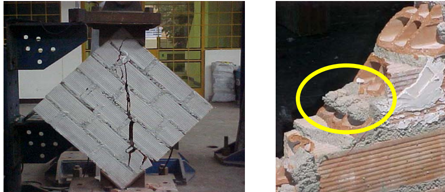
Figure 3. Diagonal tension test in little wall. Right: detail of pieces of solid mortar acting as connectors.
