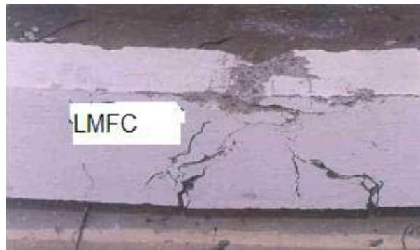
Figure 4 Typical hinged beams-failure pattern under monotonic loading
