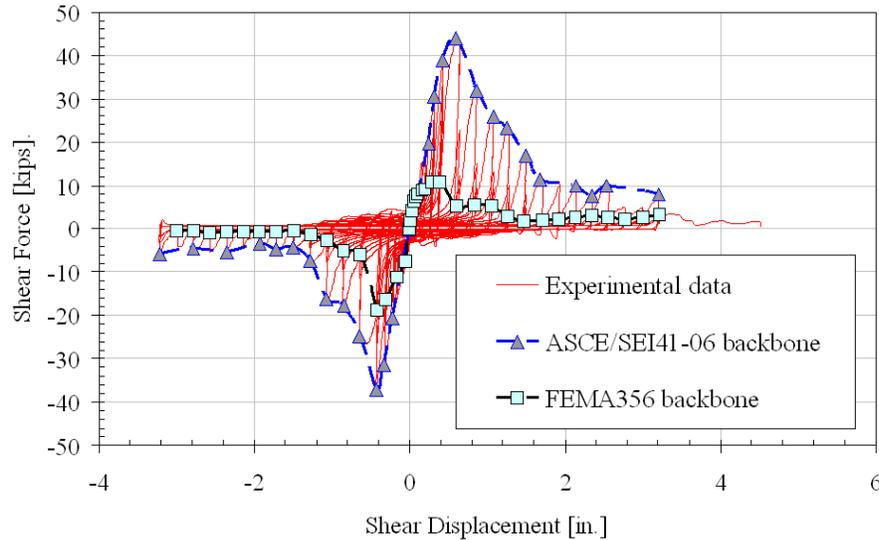
Figure 6 Backbone curve
