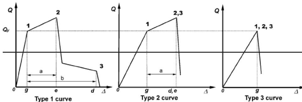
Figure 7 Component Force versus Deformation Curves [ASCE/SEI41-06]
