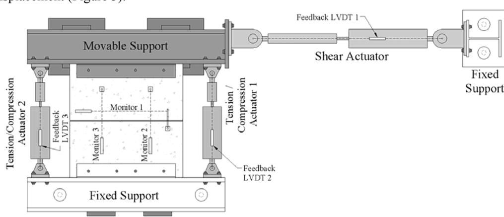
Figure 3 Multi-directional test fixture plane view
