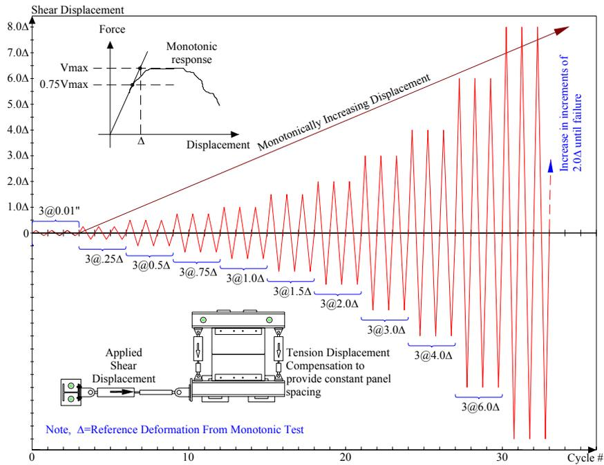
Figure 4 Shear loading protocol
