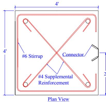
Figure 2 Supplemental reinforcement layout and construction details
