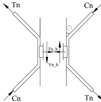
Figure 1 Truss model of double-tee connection
