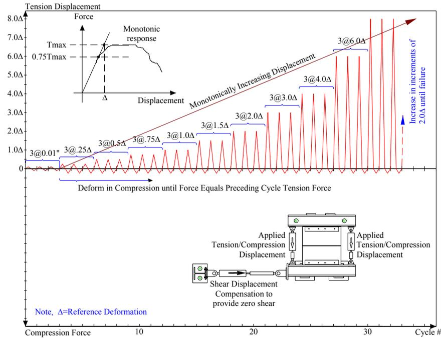
Figure 5 Tension/Compression protocol
