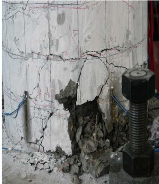
Fig. 4 Crushed concrete at the bottom end of Tube1
