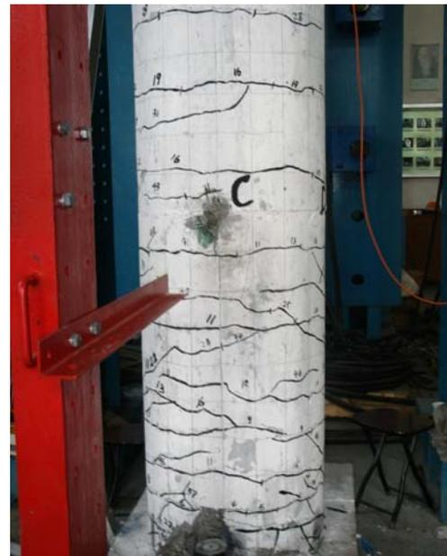
Fig. 3 Crack pattern for Tube1
