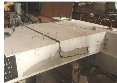
(b) North side after failure
