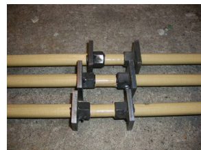
Photo 1 Fixing plates of de-bonded vertical rebar
