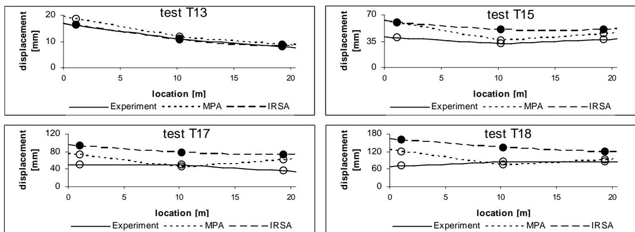
Figure 7. Comparison of maximum displacements obtained by the multimode methods and measured
