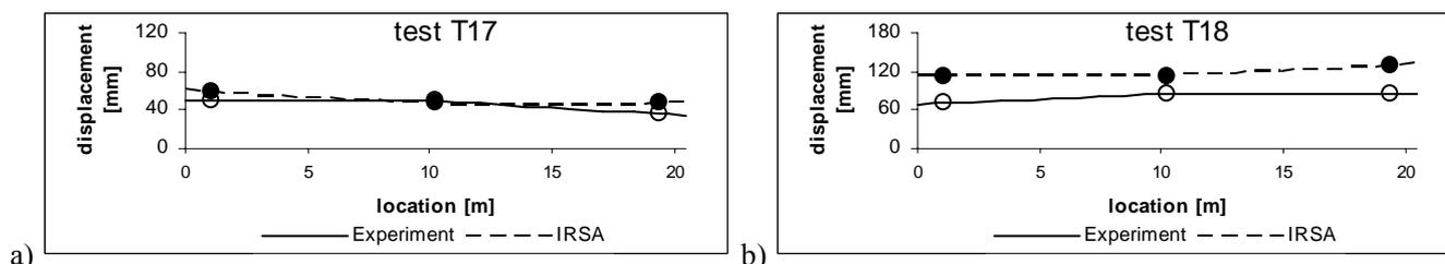
Figure 9. Displacements calculated by IRSA after the modifications of the a) damping b) ratio of the stiffness of the side bents in the test T18
