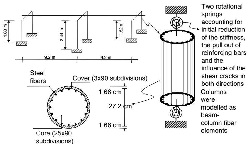
Figure 4. Analytical model of the bridge
