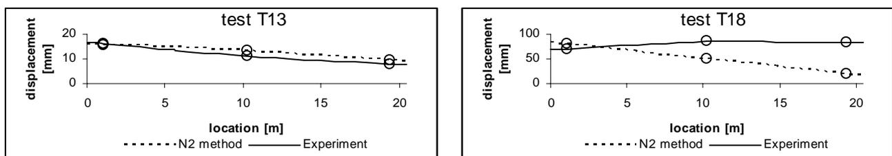
Figure 6. Displacements calculated by the N2 method and displacements measured during the experiment
