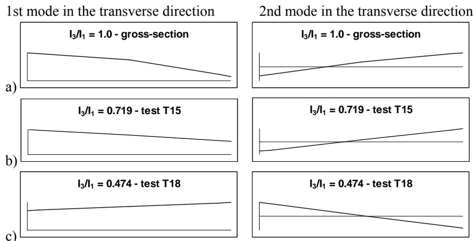
Figure 5. Changes of the mode shapes depending on the ratio of the stiffness of the bents B1 and B3
