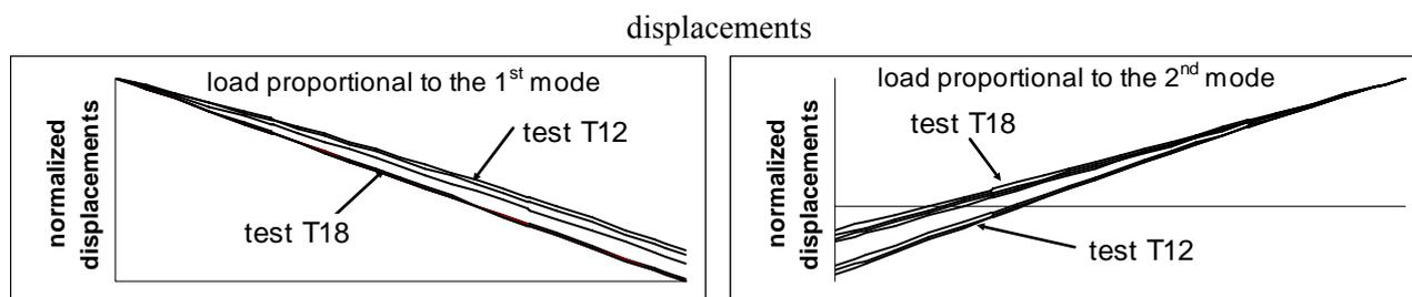
Figure 8. Normalized displacements of the bridge calculated with the MPA
