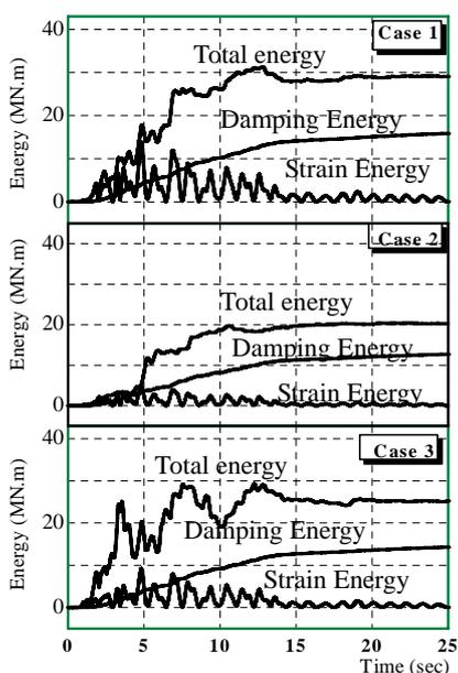
Fig. 7 Input energy to the tower
