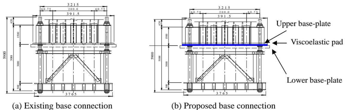
Fig. 2 Details of steel tower base connection (mm)
