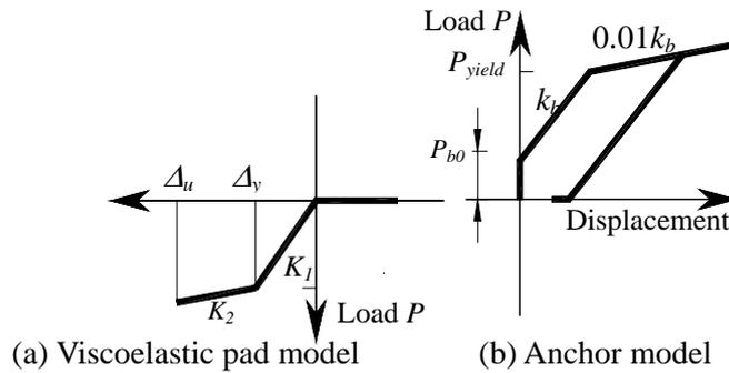
Fig. 4 Base connection components numerical models
