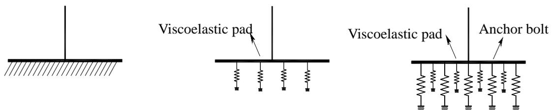
(a) Fixed base model      (b) Viscoelastic pad model      (c) Pad with anchor model
