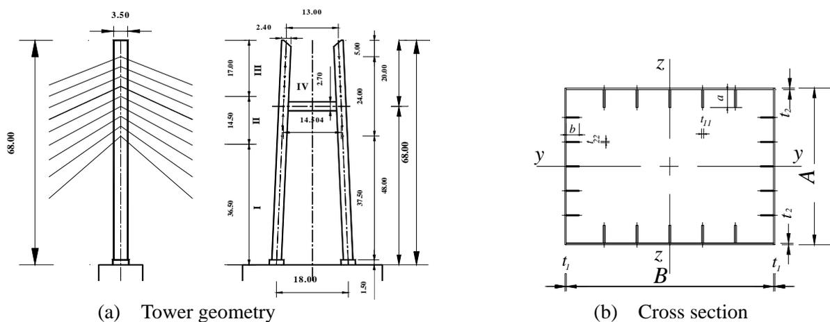
Fig. 1 Steel tower of cable-stayed bridge
