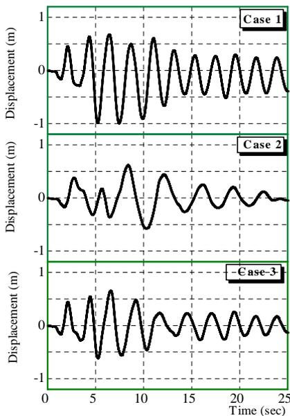
Fig. 5 Displacement time history at tower top
