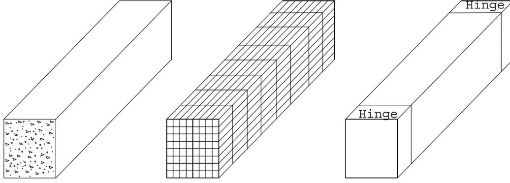
Concrete Component      Fiber Element Model      Plastic Hinge Model
