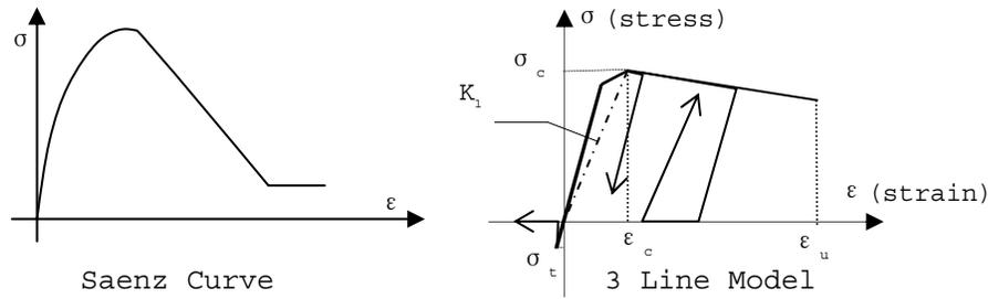
Fig. 2. Stress-Strain Model of Concrete
