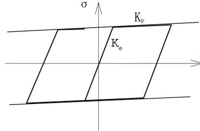
Fig.1 Stress-Strain Model of Steel
