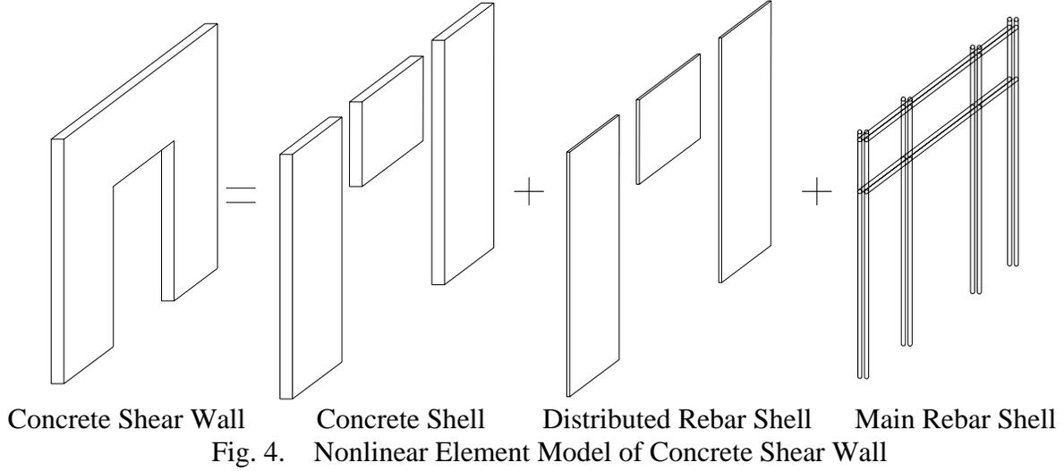
The research object of this ‘macro-shear wall element’ was the shear wall with hole, so this paper gave some methods to deal with it. This paper use ‘block integral’ shown in expression (9), and reduce shell stiffness shown in Fig. 5, expression (10)
