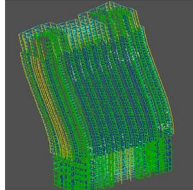
Fig.19 100,000 DOF shear wall building
