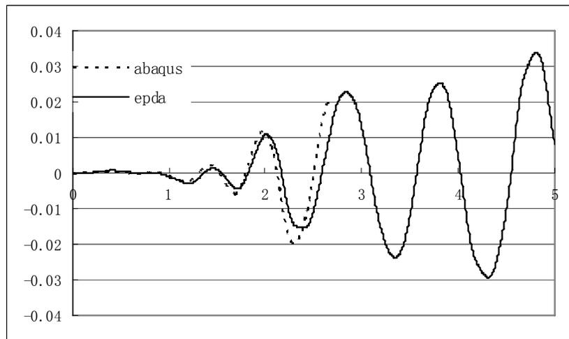
Fig. 10. Displacement time history of 10 layer concrete shear wall
