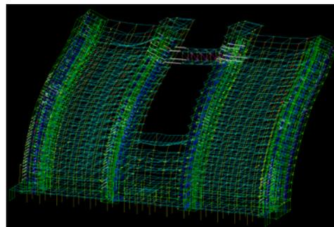
Fig. 13 Building with Isolators in corridor
