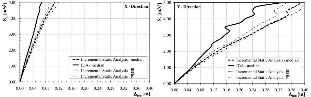
Figure 6 – Comparison between Incremental Static and Dynamic Analysis.
