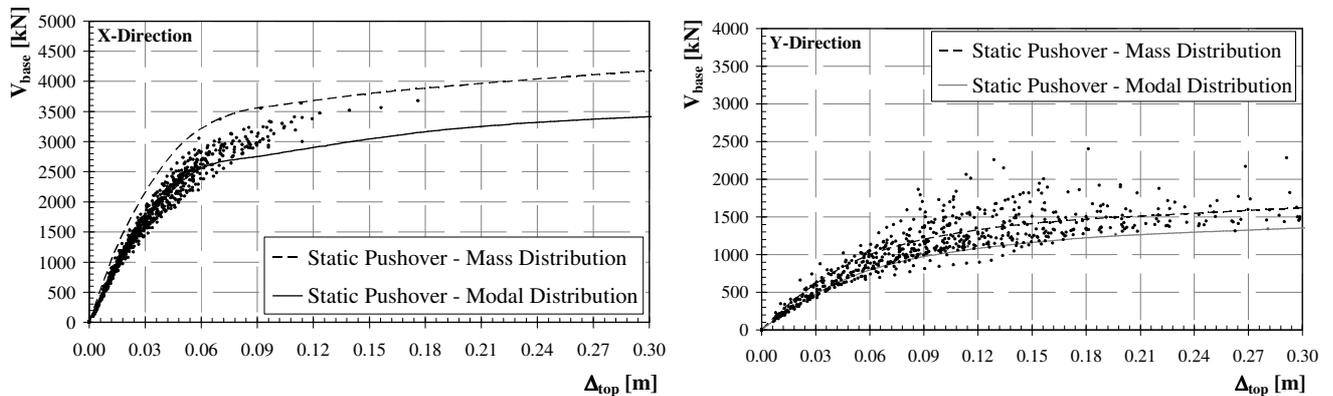
Figure 3 – Capacity curves obtained through Static and Dynamic Pushover Analysis.
