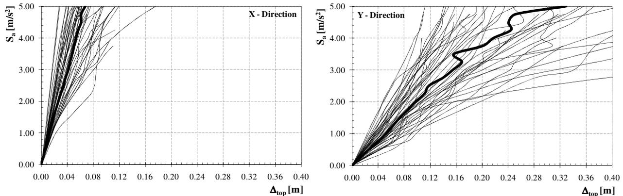
Figure 4 – Incremental Dynamic Analyses: 45 accelerograms and median value
