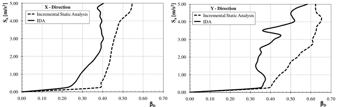
Figure 7 – Comparison between Static and Dynamic Analysis in terms of dispersion parameter  $\beta_D$ .
