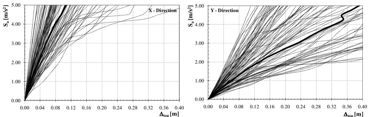
Figure 5 – Incremental Static Analysis: 45 accelerograms and median value
