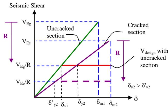
Figure 3. Relation between shear and lateral displacement
