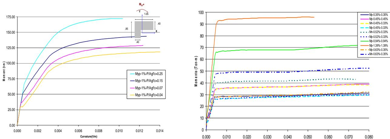
Figure 5. (a) L column (p= 1%, Y axis) Variable axial load. (b) Rectangular beam. Variable steel ratio
