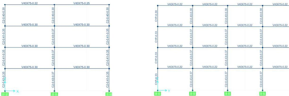
Figure 6. Frame B (X direction) and Frame 2 (Y direction). Reduction factors in beams and columns.
