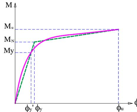
Figure 1. Moment-curvature relationship and bilinear approximation
