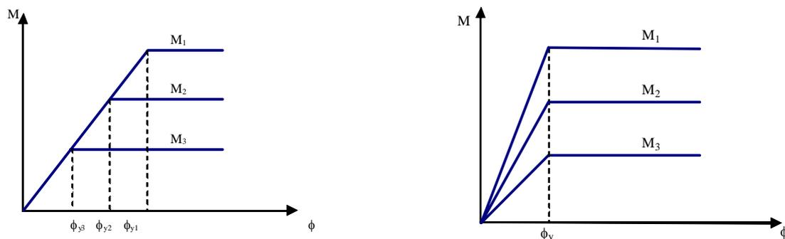
Figure 2. (a) Stiffness independent of strength. (b) Stiffness depending on strength. Constant yield curvature
