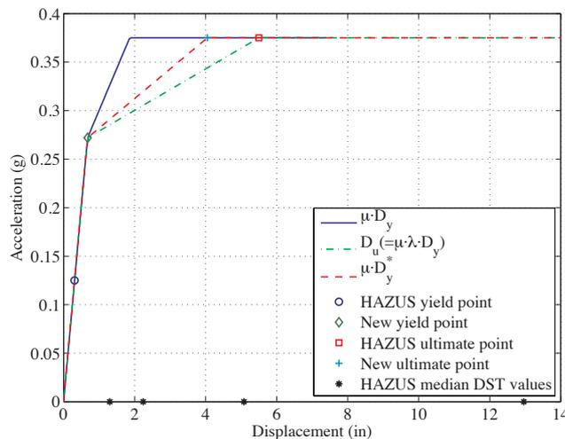
Figure 6 Capacity curves with various ultimate points
