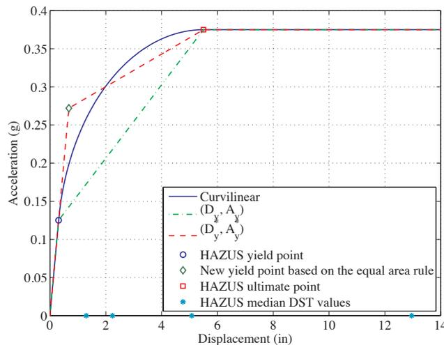
Figure 5 Capacity curves with various yield points
