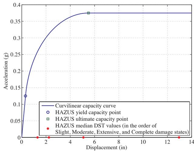
Figure 2 Curvilinear HAZUS capacity curve for a moderate-code low-rise steel moment resisting frame building
