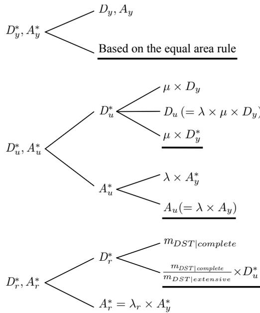
Figure 4 A tree illustrating options for determining multilinear capacity curve parameters
