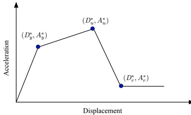
Figure 3 Multilinear capacity curve
