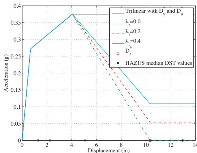
Figure 7 Capacity curves with various residual capacity points
