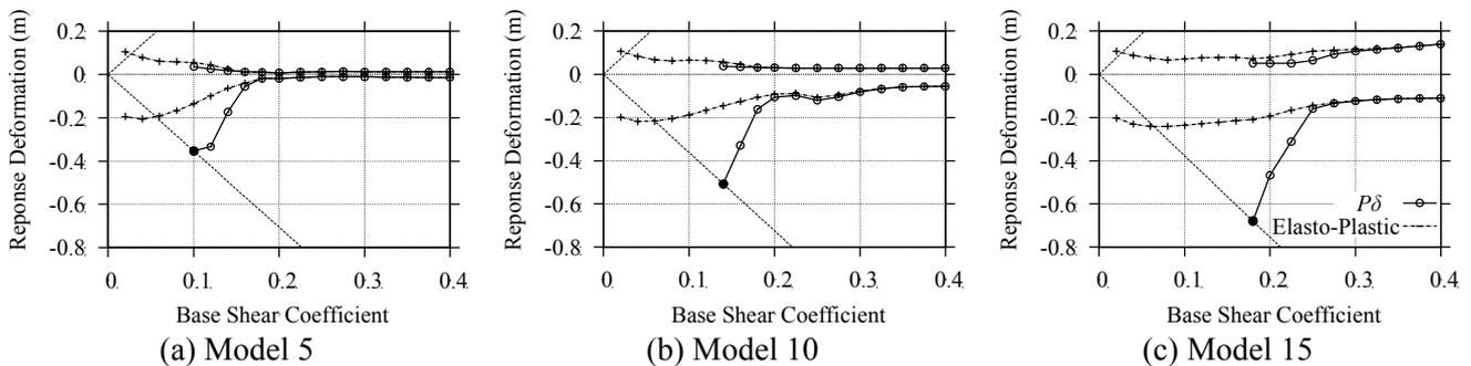
Figure 5 Relation between Base Shear Coefficient and Positive and Negative Response Deformation subjected to *Symmetric* Motion
