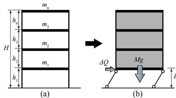
Figure 2  $P-\delta$  Effect of Multi Degree of Freedom System
