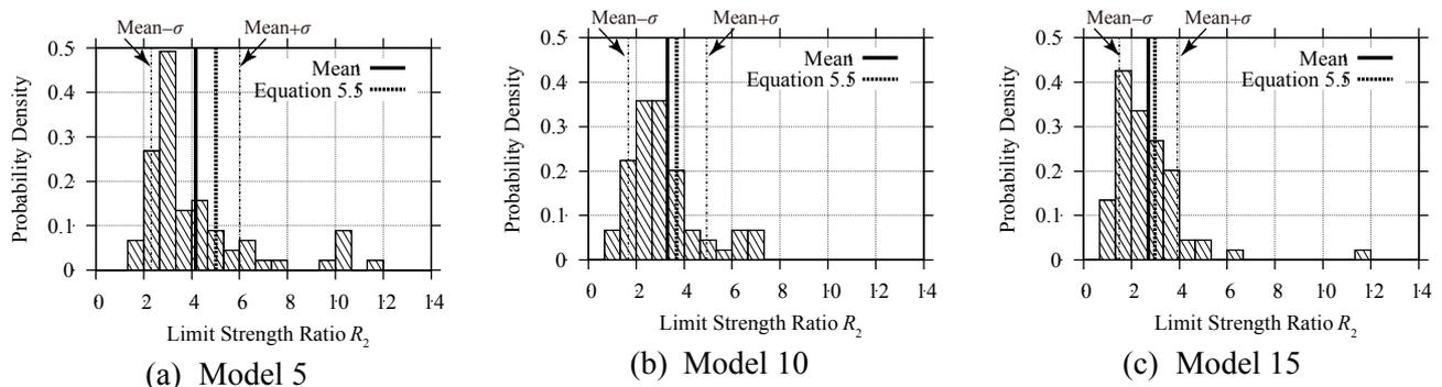
Figure 13 Histogram of Limit Strength Ratio  $R_2$  computed with 68 Real Ground Motions
