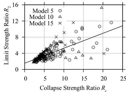
Figure 12 Relation between Collapse Strength Ratio  $R_c$  and Limit Strength Ratio  $R_2$
