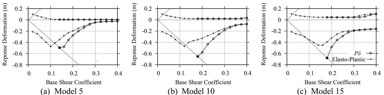
Figure 6 Relation between Base Shear Coefficient and Positive and Negative Response Deformation subjected to *Asymmetric* Motion
