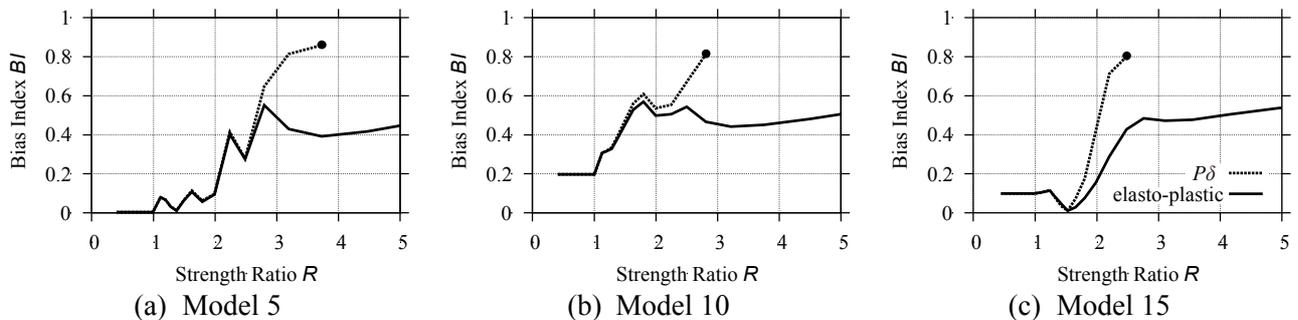
Figure 7 Strength Ratio  $R$  – Bias Index  $BI$  subjected to *Symmetric* Motion
