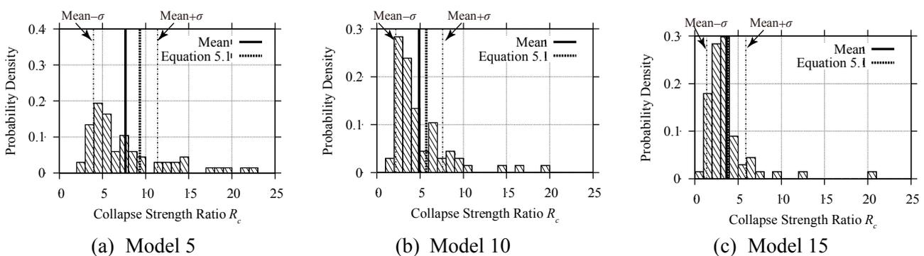
Figure 9 Histogram of Collapse Strength Ratio  $R_c$  computed with 68 Real Ground Motions
