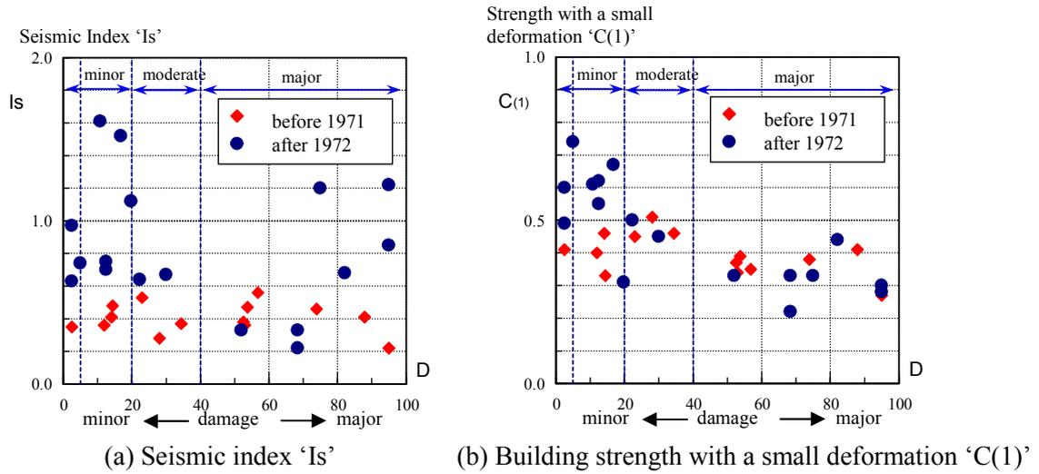
Fig 1. Relationship between structural performance and damage
