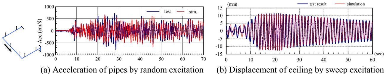
Fig 3. Comparison of test results and simulation
