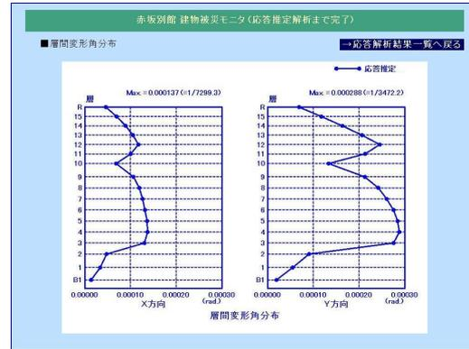
Fig 5. Observed acceleration at building A      Fig 6. Estimated maximum story drift angle
