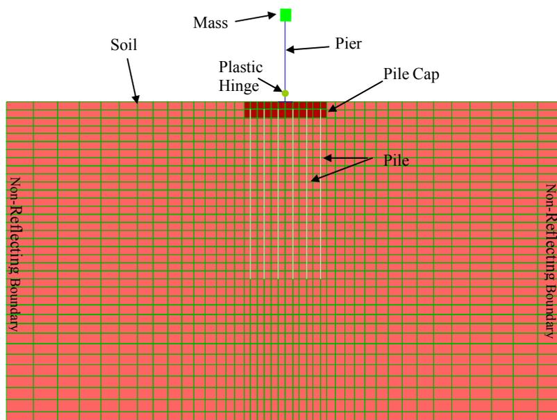
Figure 1: Geometry of the FLAC model (top 30 m of soil)
