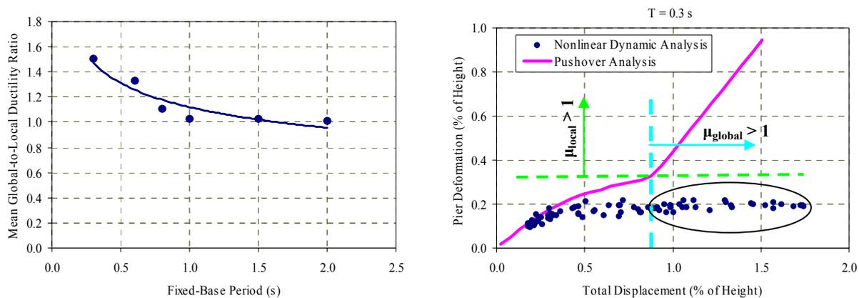
Figure 5: (a) Mean ratio of the global ductility to the local ductility factors; (b) Pier deformations vs. total displacements: comparison of results from pushover and nonlinear dynamic analyses of piers with  $T = 0.3$  s
