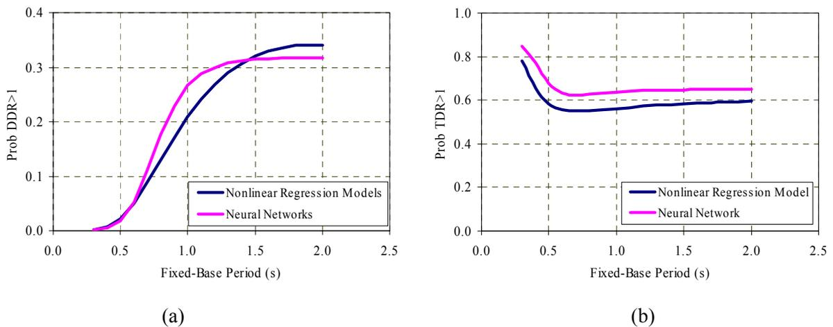
Figure 3: (a) Probability of  $DDR > 1.0$ ; (b) Probability of  $TDR > 1.0$  as functions of the fixed-base period
