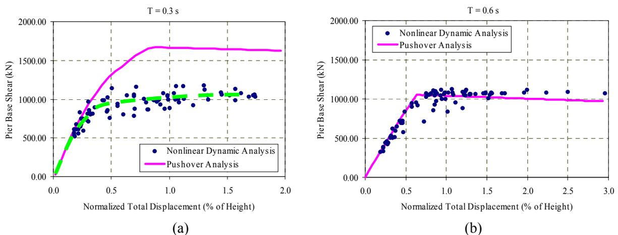
Figure 4: Comparison of the force-displacement relationships (including SSI) obtained from pushover and nonlinear dynamic analyses of the piers with (a)  $T = 0.3$  s and (b)  $T = 0.6$  s
