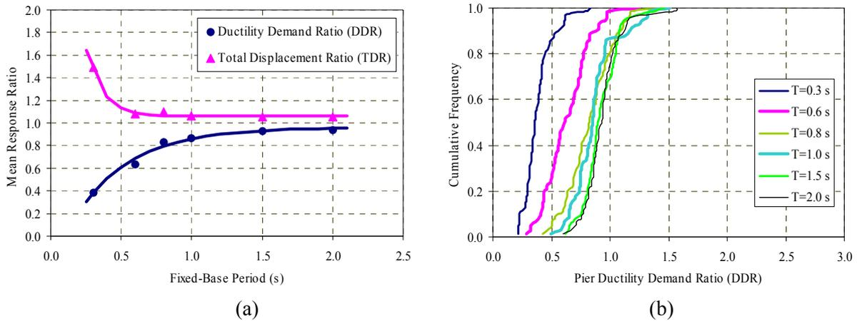
Figure 2: (a) Mean response ratios DDR and TDR; (b) Distributions of pier Ductility Demand Ratios (DDR)
