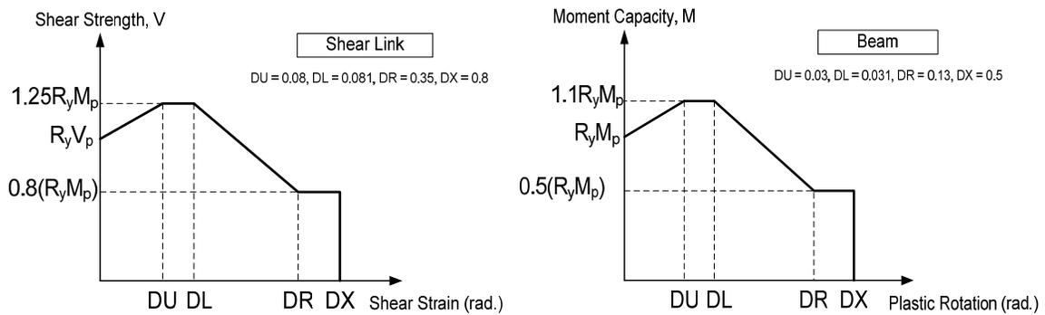
Figure 2 Member strength envelopes for modeling: shear link and beam
