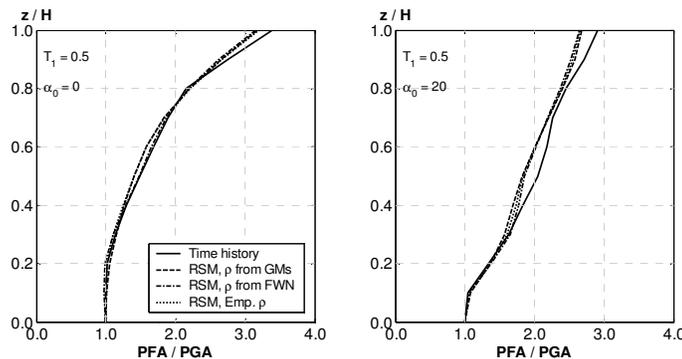
Figure 6 – comparison of peak floor acceleration profiles, time history analysis, FWN and GM, absolute acceleration method for  $T_1 = 0.5$  s
