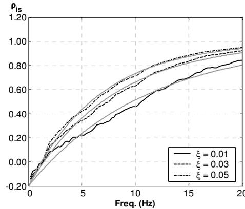
Figure 4 – average and fitted correlation between ground acceleration and SDOF absolute acceleration
