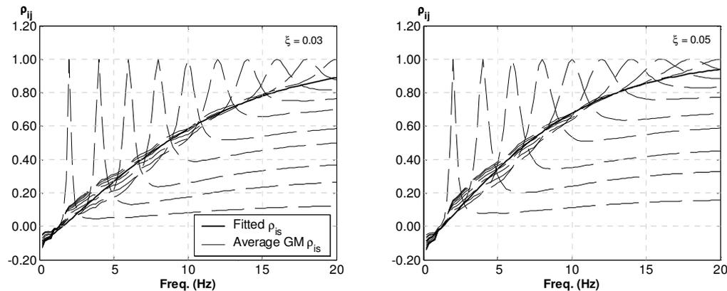
Figure 5 – average and fitted correlation between SDOF absolute accelerations
