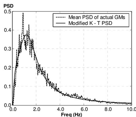
Figure 1 – Average power spectral density of ground motions and fitted modified K-T PSD.
