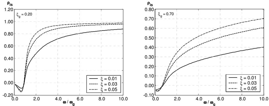
Figure 2 - correlation function between ground acceleration and SDOF system absolute acceleration for wide and narrow band ground motions
