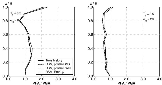
Figure 7 – comparison of peak floor acceleration profiles, time history analysis, FWN and GM, absolute acceleration method for  $T_1 = 3.5$  s
