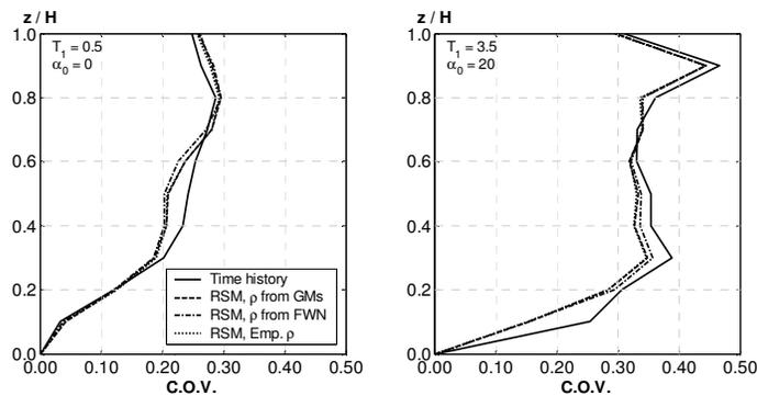
Figure 8 – coefficients of variation between time history results, GM and fitted results, absolute acceleration method
