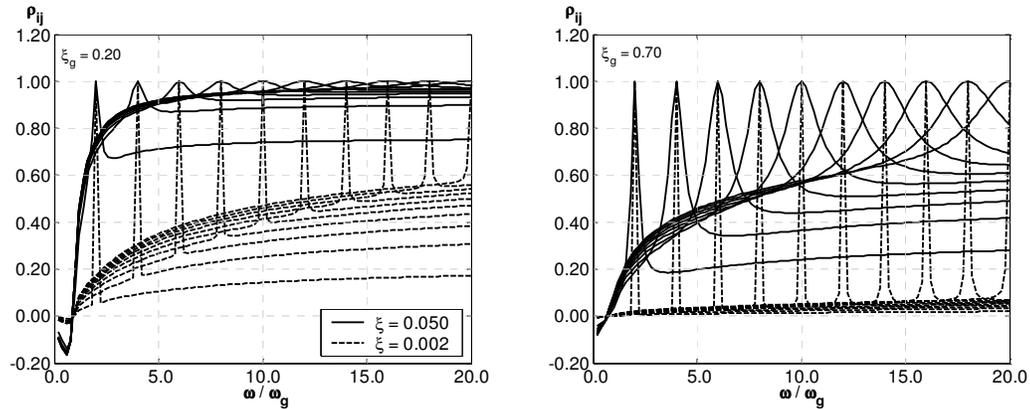
Figure 3 - correlation functions between SDOF absolute accelerations for wide and narrow band ground motions with two values of damping for the structure
