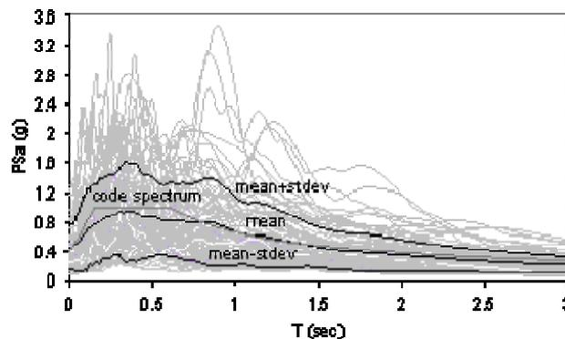
Figure 5. Acceleration response spectra for the 96 ground motion
