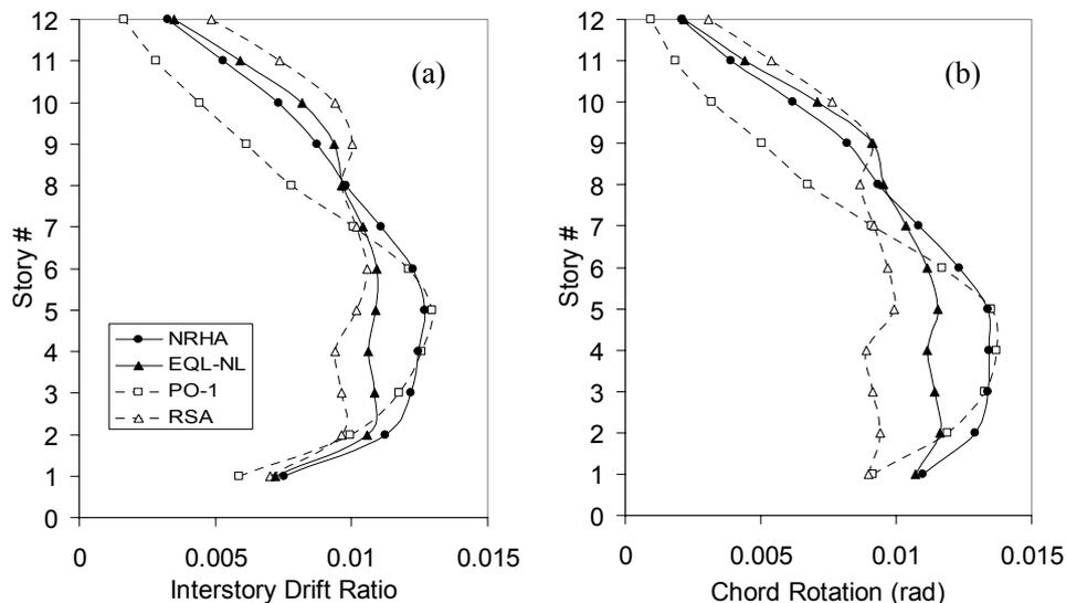
Figure 7. Median values of a) interstory drift ratios, b) beam chord rotations.
