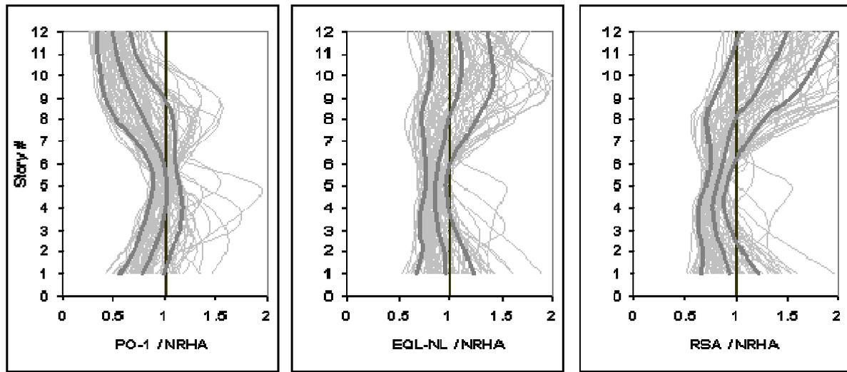
Figure 8. Interstory drift ratios of the approximate methods normalized with those of NRHA for all ground motions
