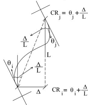
Figure 2. Definition of chord rotation at the i and j ends of a frame member
