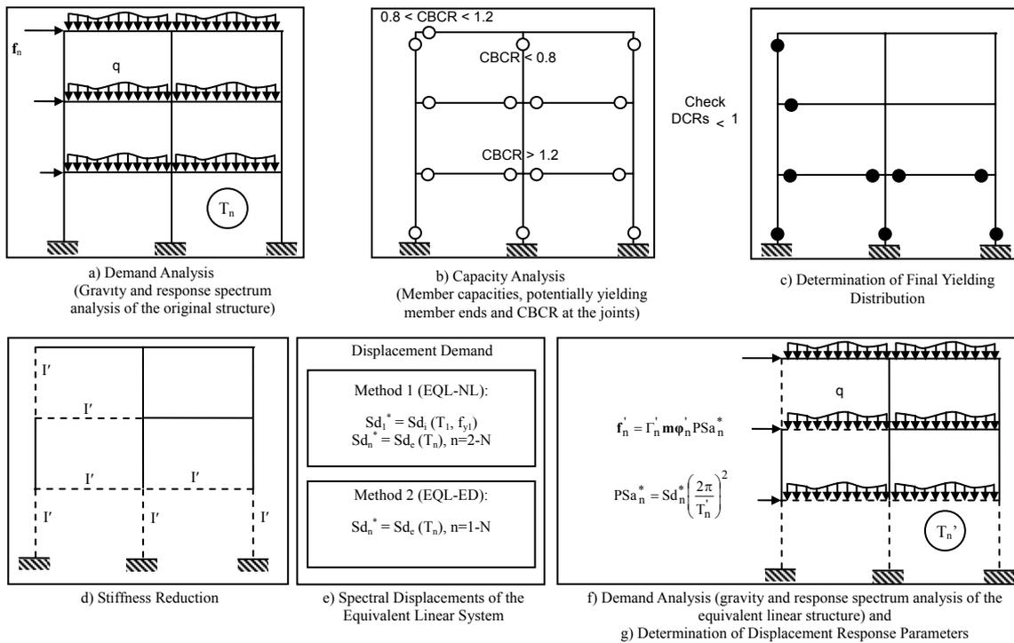
Figure 4. Schematical demonstration of the equivalent linearization procedure
