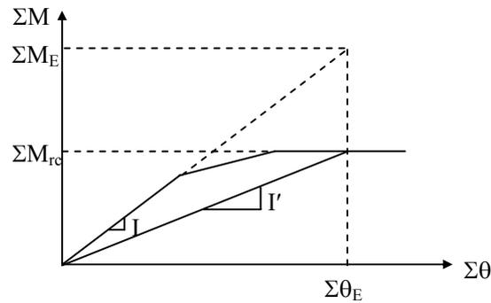
Figure 3. The variation of total end moments with total chord rotations at member-ends in the linear elastic and inelastic ranges
