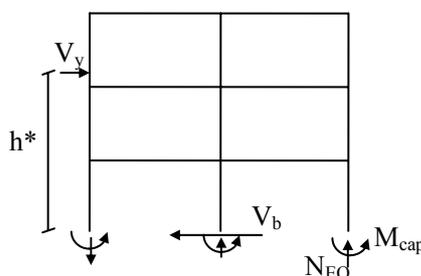
Figure 1. Calculation of base shear capacity for 2D models
