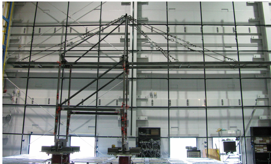
Figure 2: Completed 1:20 Scale Crane Specimen
