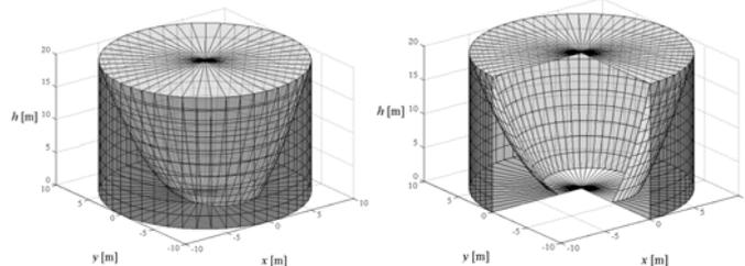
Figure 6. Three-dimensional views of portion A1 (in light grey) and of portion A2 (in dark grey) of the flat-bottom grain silo: overview and sectioned view
