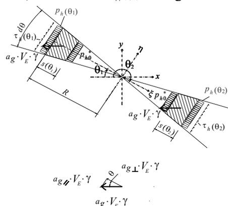
Figure 4. Vertical and horizontal actions operating on disk  $D$  and symmetrical elements  $E$  placed at different heights in the presence of additional horizontal and vertical acceleration
