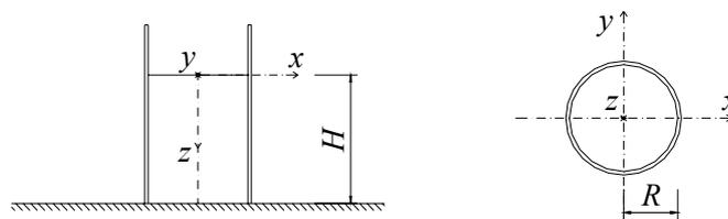
Figure 1. Geometry of a flat-bottom grain silo and reference system adopted
