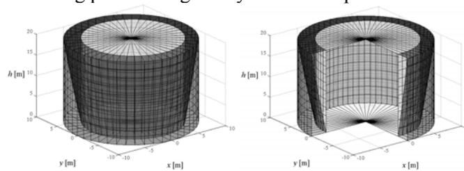
Figure 7. Three-dimensional views of portion B1 (in light grey) and of portion B2 (in medium-light grey) and of portion B3 (in dark grey) of the flat-bottom grain silo: overview and sectioned view
