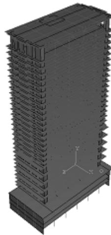
Figure 1 Three-dimensional finite model
