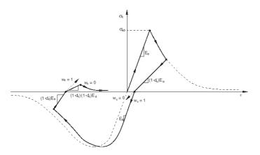
Figure 1 Concrete tension-compression stiffness restoration curve
