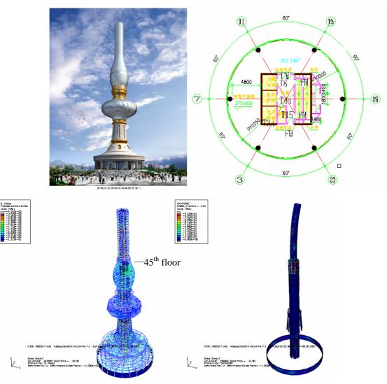
Figure 3 Three-dimensional effect, the floor plan, overall Mises stress and shear wall compression damage
