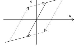
Figure 2 Steel tension-compression hysteretic curve
