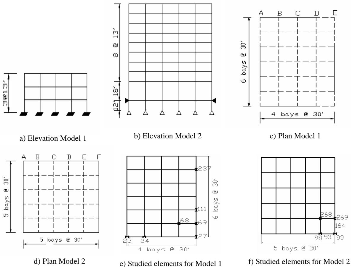
Figure 1. Elevations, plan and element location for Models 1 and 2
