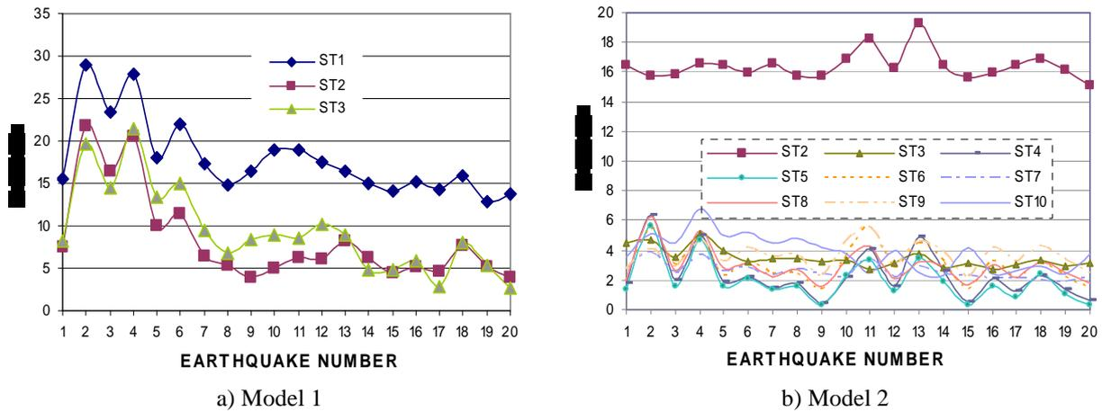
Figure 2.  $V_I$  values for Models 1 and 2 with PP connections
