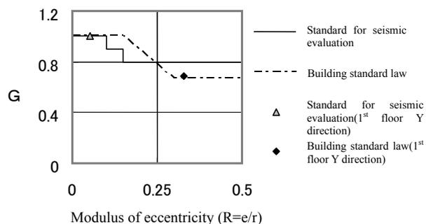
Fig.3 Relation between modulus of eccentricity and G1 value of 1<sup>st</sup> floor Y direction
