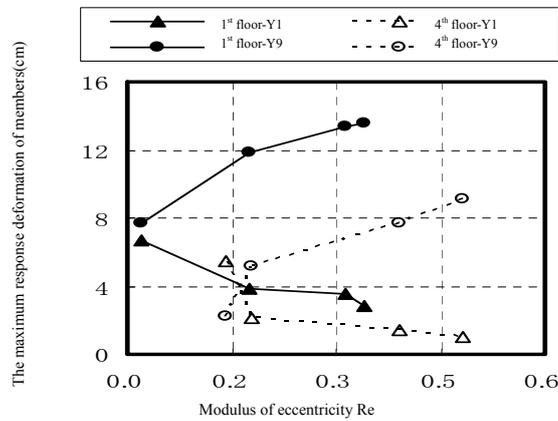
Fig. 10 Change of outmost frame response in Y direction by variation of wall position
