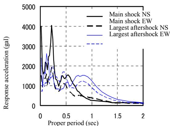
Fig.5 Acceleration spectrum of the earthquake (at Tokamachi City Hall)
