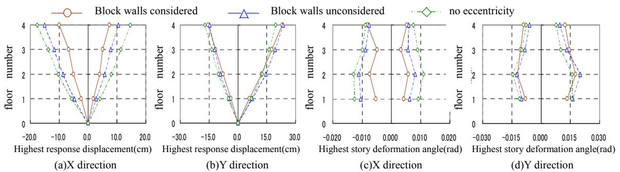
Fig.6 Effect of analytical model (maximum response displacement and maximum story deformation angle at the center of gravity in case of main shock and aftershock)
