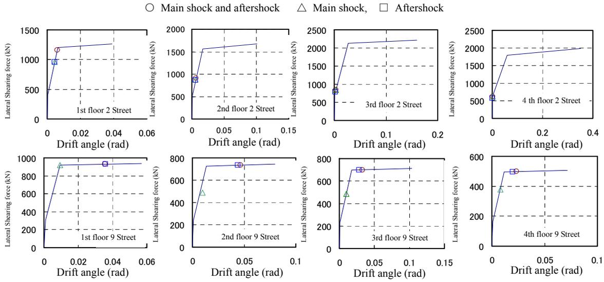
Fig.8 The maximum response of 2 Frame and 9 Frame of each floor
