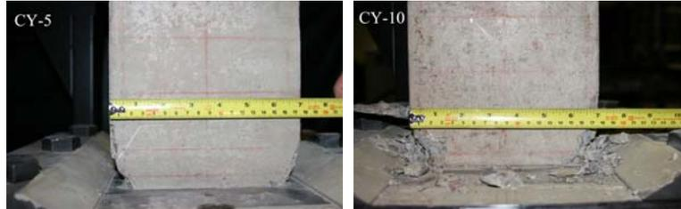
Figure 3 Crushing of rocking column edges after testing
