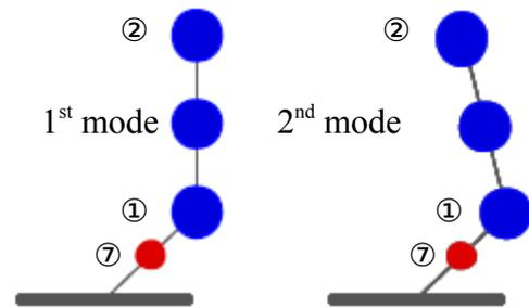
Figure 6. Graphical representation of vibration modes for base isolated building.
