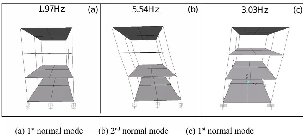
Figure 12. Vibration modes obtained from a FEM analysis for base isolated building (a) 1<sup>st</sup> normal mode and (b) 2<sup>nd</sup> normal mode, and for building without isolation (c) 1<sup>st</sup> normal mode
