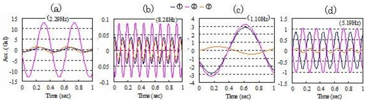
Figure 11. Waveforms obtained after filtering for building without base isolation (a) 2.29 Hz and (b) 8.28 Hz, and base isolated building (c) 1.10 Hz and (d) 5.19 Hz.
