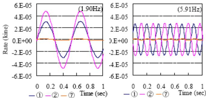
Figure 5. Waveforms for 1.90 Hz and 5.91 Hz obtained after filtering at base isolated building
