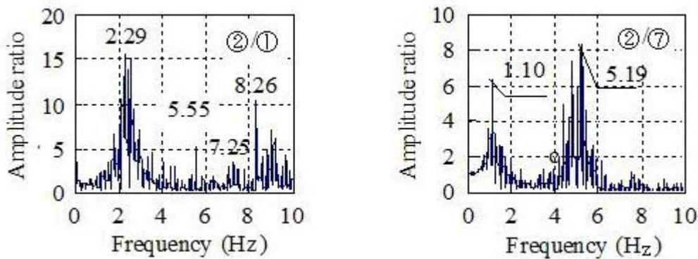
Figure 10. Transfer functions for building without base isolation (left) and base isolated building (right).
