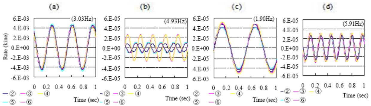
Figure 4. Waveforms obtained after filtering for building without base isolation (a) 3.03 Hz and (b) 4.93 Hz, and base isolated building (c) 1.90 Hz and (d) 5.91 Hz.
