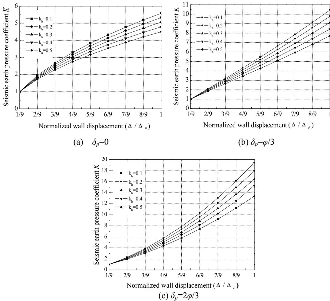
Figure 2 Seismic earth pressure coefficients at the passive side
