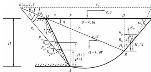
Fig. 1. Dynamic intermediate soil wedge with curved surface
