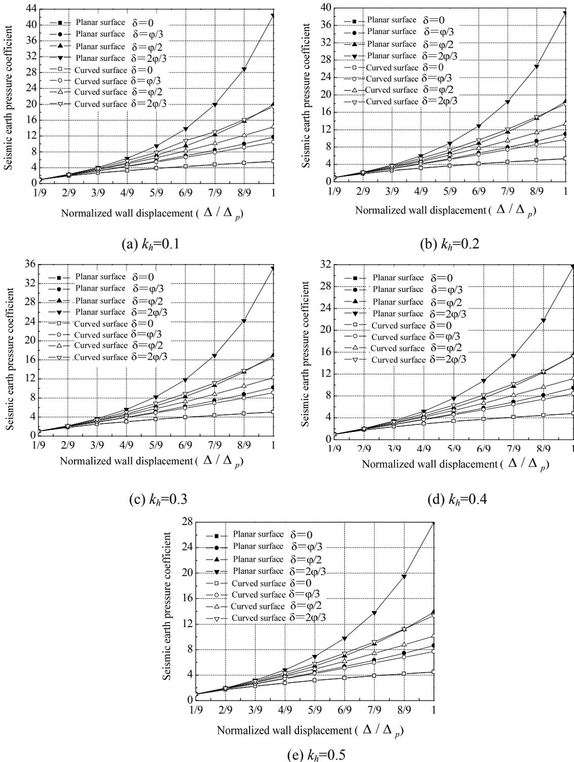
Fig 3 Comparison of seismic earth pressure coefficients for  $\varphi=45^\circ$ ,  $\alpha=0^\circ$ ,  $k_v=0$
