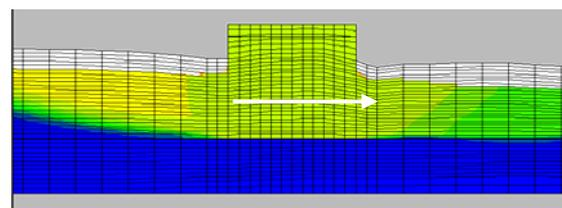
Figure 8: Failure Surface of Base Condition
