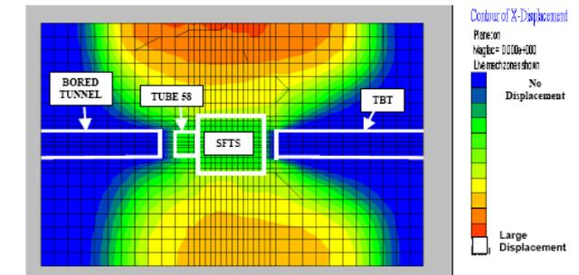
Downslope Failure Pattern at Tube-Level Elevation (Elevation -80ft)
