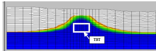
Downslope Failure Pattern along the Transverse Cross-Section (90 ft east of SFTS)
