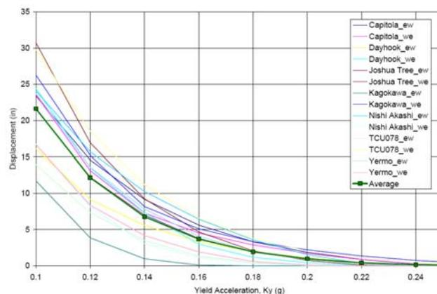
Figure 15: Yield Acceleration vs. Displacement of SFTS
