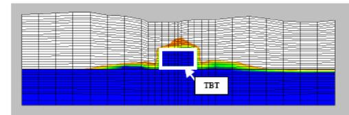
Downslope Failure Pattern along the Transverse Cross-Section (20 ft east of SFTS)
