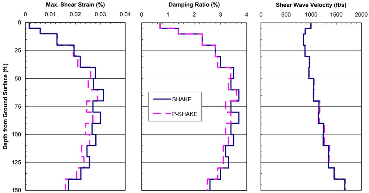
Figure 5 Comparison of Maximum Shear Strains and Strain-Compatible Soil Property Profiles
