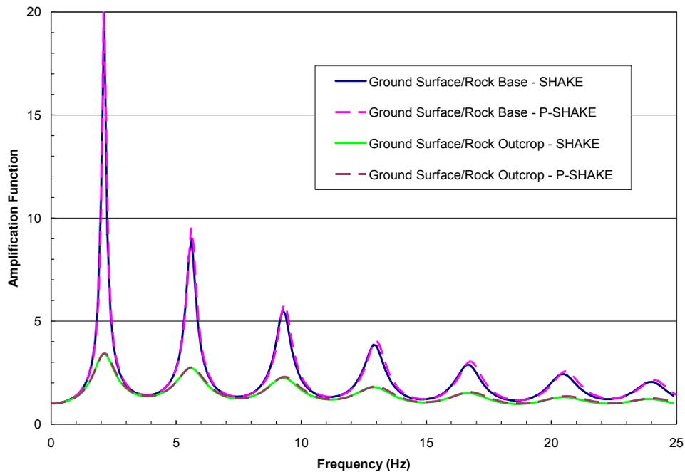
Figure 8 Comparison of Amplification Functions Between Motions at Ground Surface and at Rock Base
