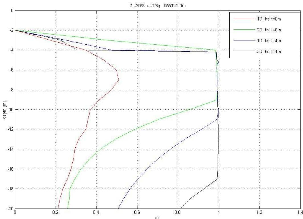
Figure 1 The effect of a silt seam on a sand soil with 30% of relative density
