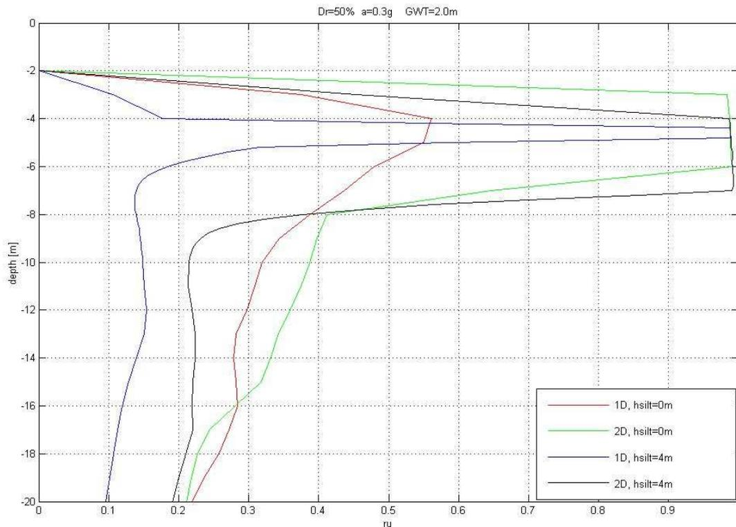
Figure 2 The effect of a silt seam on a sand soil with 50% of relative density
