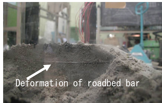
Figure 6 Case4 After Vibration Experiment (cross-section)
