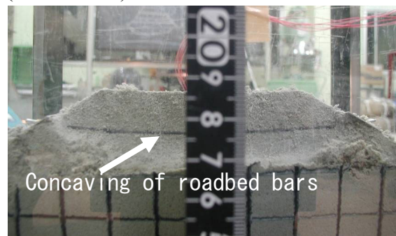
Figure 8 Case5 After Vibration Experiment (cross-section)
