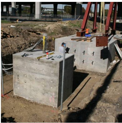
Figure 2: Single pile specimen at the test site
