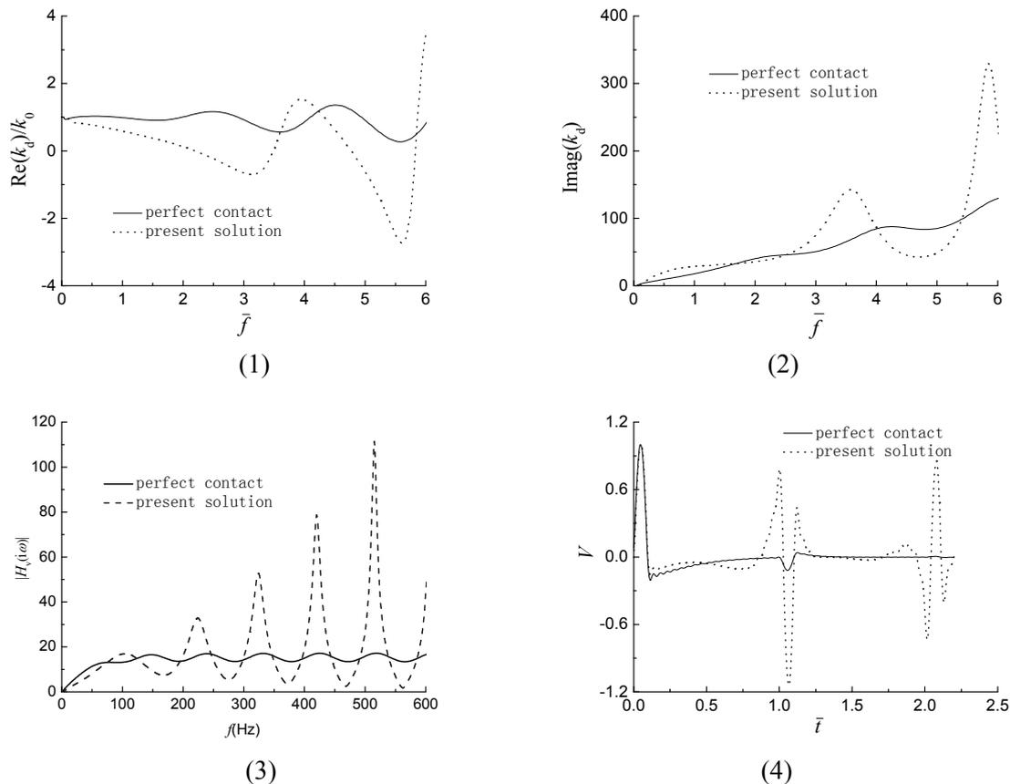
Figure 2 Comparison of pile dynamic response for different model
