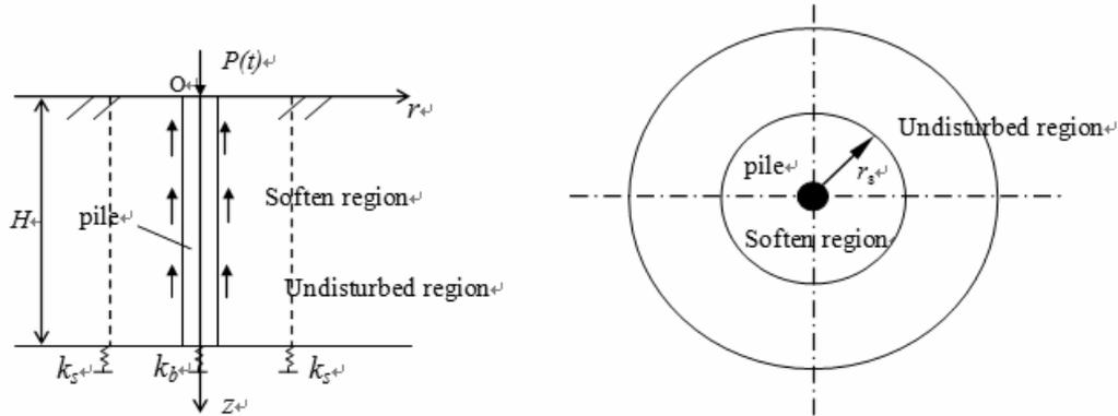
Figure 1 Sketch of soil-pile interaction
