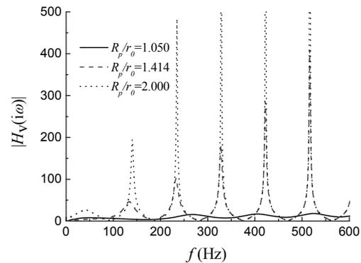
Figure 3 Effects of equivalent modulus on pile admittance    Figure 4 Effects of radius ratio on pile admittance
